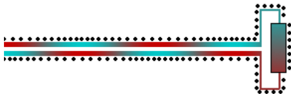
Fig:1 Schematic showing how a wave flows down a lossless transmission
