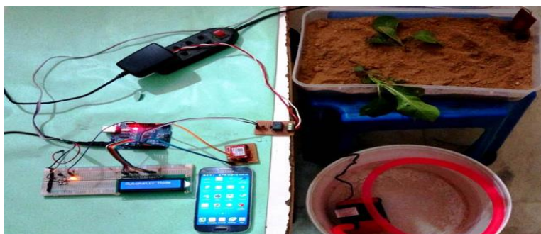
Set up of Soil Moisture Sensor
